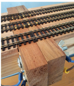
A detail photo of how 2 joining 'blocks' fit together, locate track and pass power between modules
