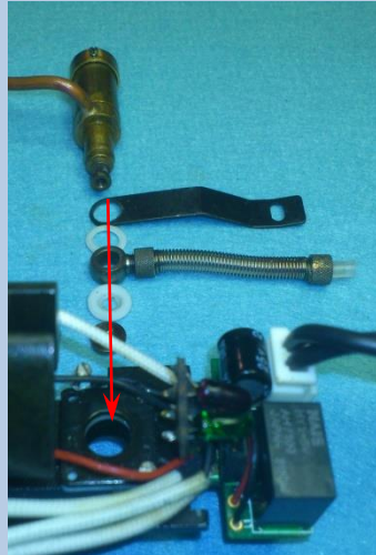
The relief valve chamber. Showing how the tender drawbar, steam pipe and its banjo coupling are assembled onto the relief valve.
