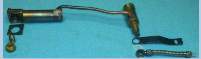
Above shows the relief valve chamber on the right with the super heater chamber on the left both connected with a pipe soldered to each.
